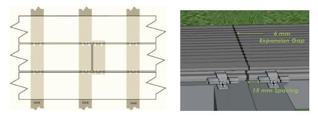
For the first board, install to the baton as detailed above. For the second board, attach a second board on a second baton/joist – as above diagram.
