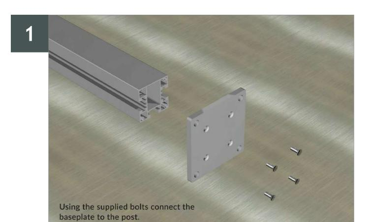
Attach the post to the ground (or decking) carefully. If installing onto SAiGE decking ensure solid boards are used measuring the required centres (1.8m).
