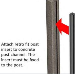
insert to concrete post channel. The insert must be fixed to the post.
