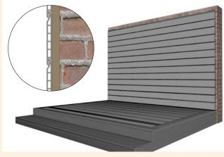
Slot the second board into place and repeat the fixing process, until you reach the desired height.
